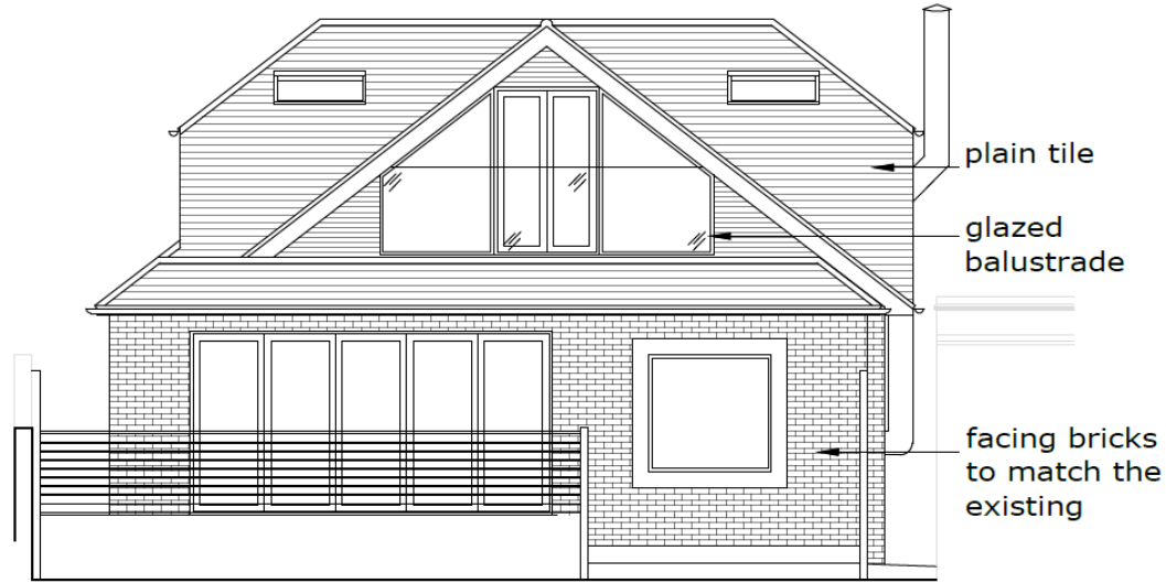
proposed west elevation 1:100
